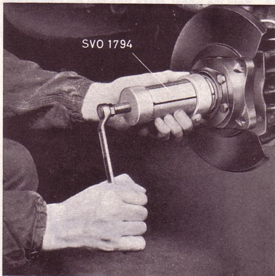
Fig. 26. Removing the inner bearing
