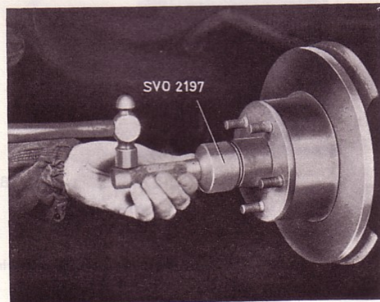
Fig. 24. Removing the grease cap
